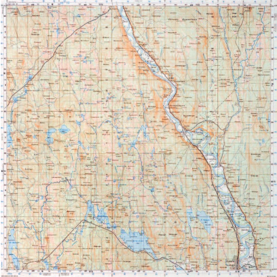
Figure 6-3. Topographic map (with a part of the river Klarälven) of the kind issued in the second half of the 1900s, based on renewed triangulation (combined with aerial photography).
