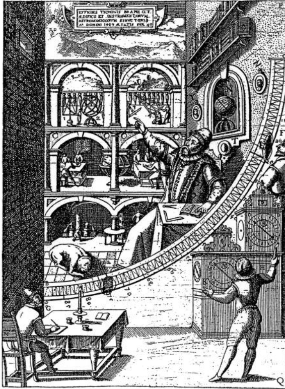
Figure 3-2. The large quadrant in Uraniborg, used for determining the latitude of the observatory from the altitudes of stars. The persons in the foreground are observers; the area above the quadrant itself is covered by a wall painting. (Brahe, 1598.)
