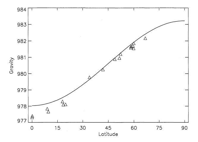
*Figure 3.* Normal gravity curve according to GRS 1980 compared with the gravity observations of Table 1.
