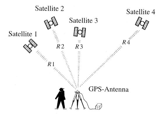
Figure 1. The basic idea of the Global Positioning System, GPS (from Seeber, 2003).
