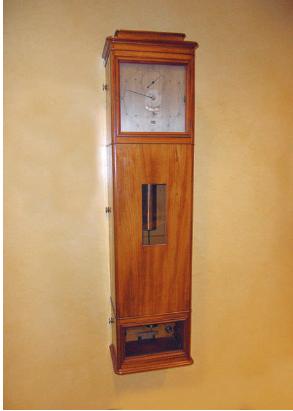
Figure 5-10. The pendulum clock of Celsius, constructed for him by Graham in London in 1741 and used by Celsius for determining the value of gravity at the latitude of Uppsala.
