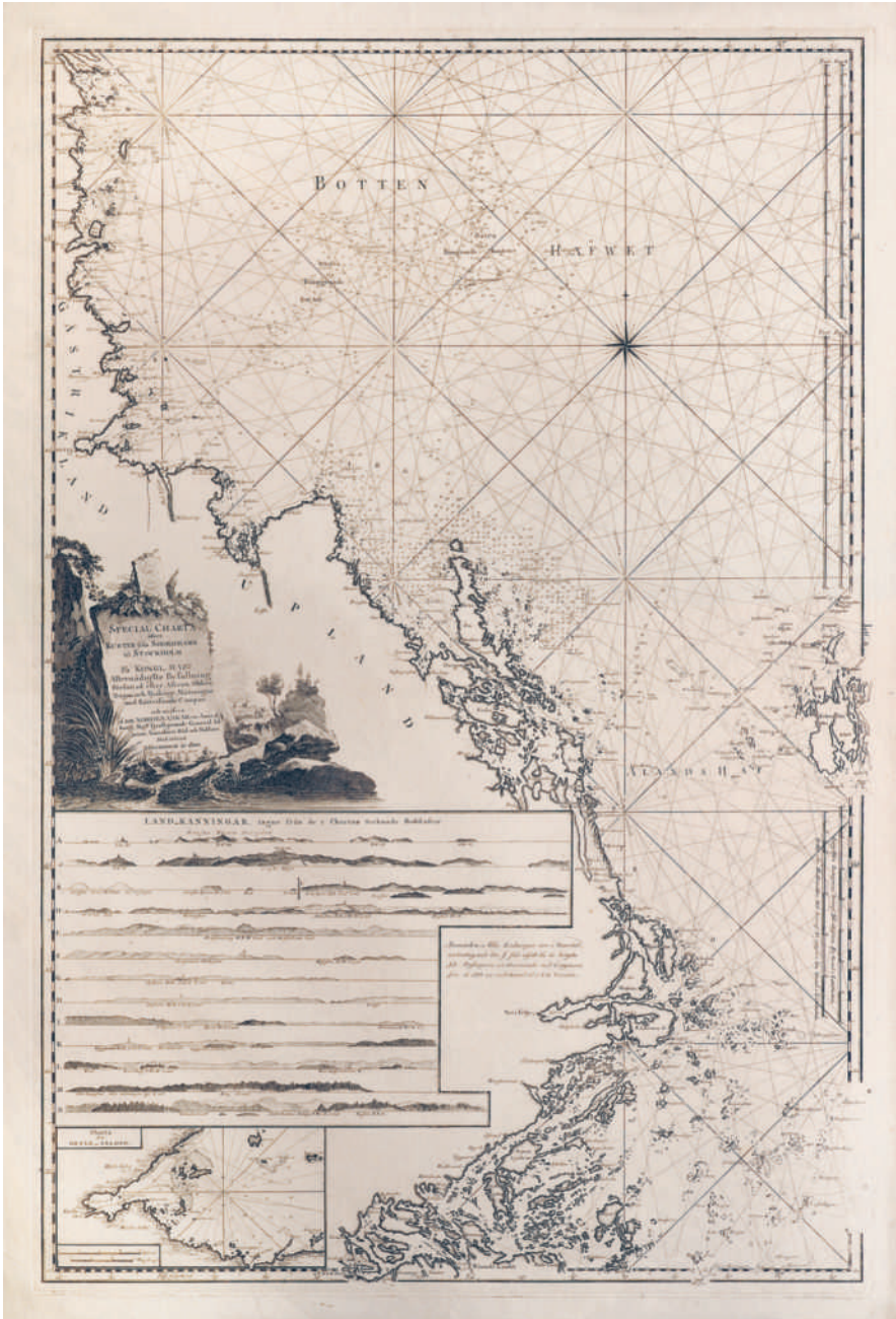
Figure 5-9. Accurate nautical chart of the Åland Sea and its surroundings based on triangulation campaigns initiated by the early works of Celsius and Gadolin.
