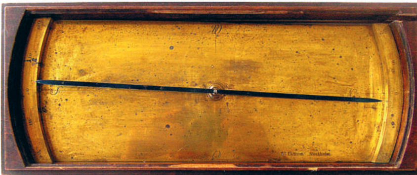
Figure 5-19. The contemporary copy of the long magnetic needle (compass) ordered by Celsius from Graham in London in 1736 and used for studying changes in the magnetic field.
