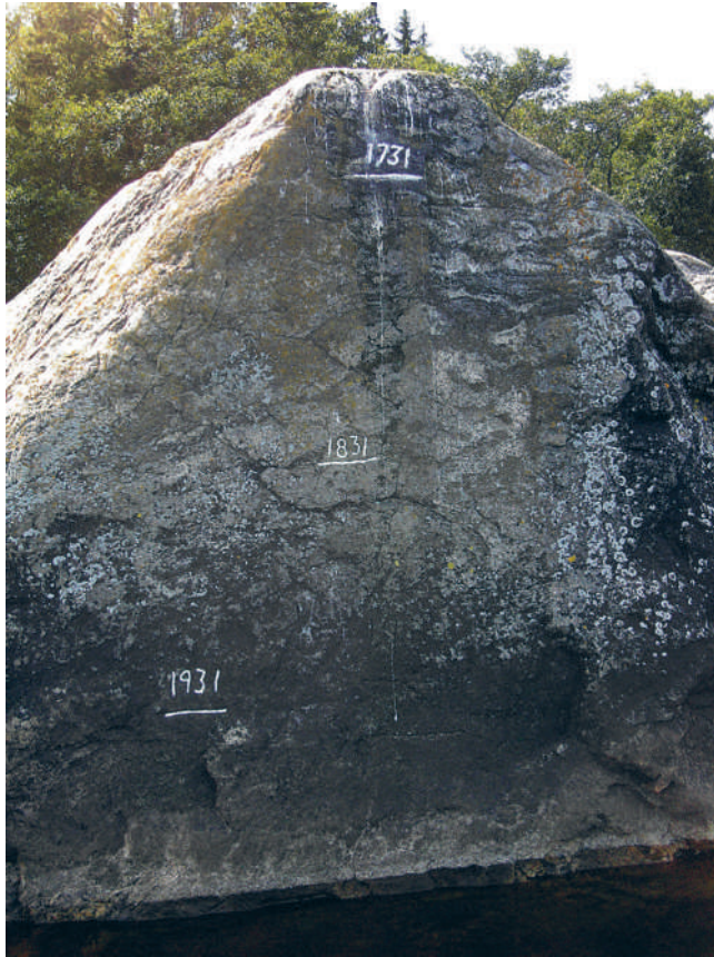
Figure 5-14. The seal rock at Lövgrund today. Celsius' mean sea level mark of 1731 at the top, later marks for each centenary below, illustrating the gradual land uplift. There will be room for a last mark in 2031.
