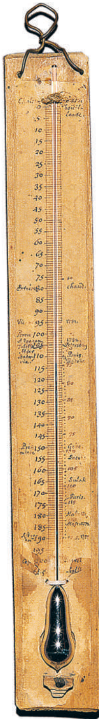
Figure 5-16. Celsius' experimental thermometer sent to him from Delisle in St. Petersburg. Delisle's temperature scale to the left with Celsius' new temperature scale, completed in 1741, added to the right.
